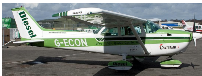
Cessna Centurion 1.7 com motor diesel
